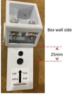
Bolt drive onto other end square mounting frame with the 2 x 8mm bolts through square tube mounting and 3 x  $^{2}$  6mm bolts through gearbox
